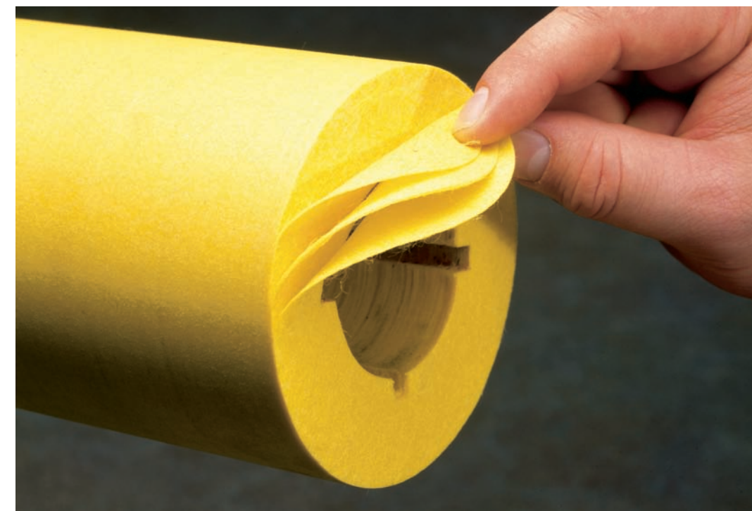
Individual discs of non-woven synthetic fiber bonded together with a tough flexible adhesive for a unique combination of characteristics – resiliency, gouge resistance, self-healing, porosity, and absorbency.
